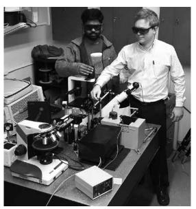
Conducting time-resolved fluorescence measurements in the Photonics Lab of the Department of Electrical and Computer Engineering at North Dakota State University.
