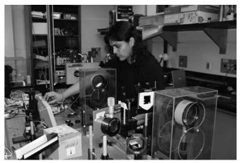
SDSU undergraduate Luis Guerrero is working on an optical pattern recognition (Fourier transform) optical system.
