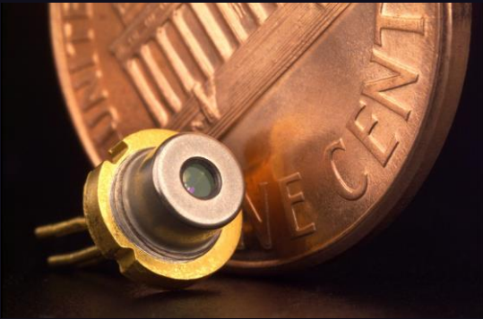
A 5.6 mm 'closed can' commercial laser diode, such as those used in a laser pointer.
