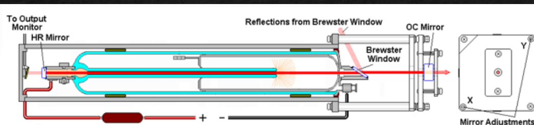
HeNe Laser Tube with Internal HR and Brewster Window with External OC
