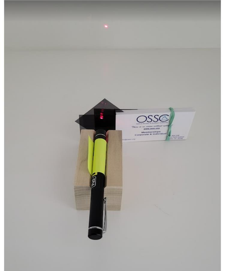
Laser with P(h+ v + 45) filters
