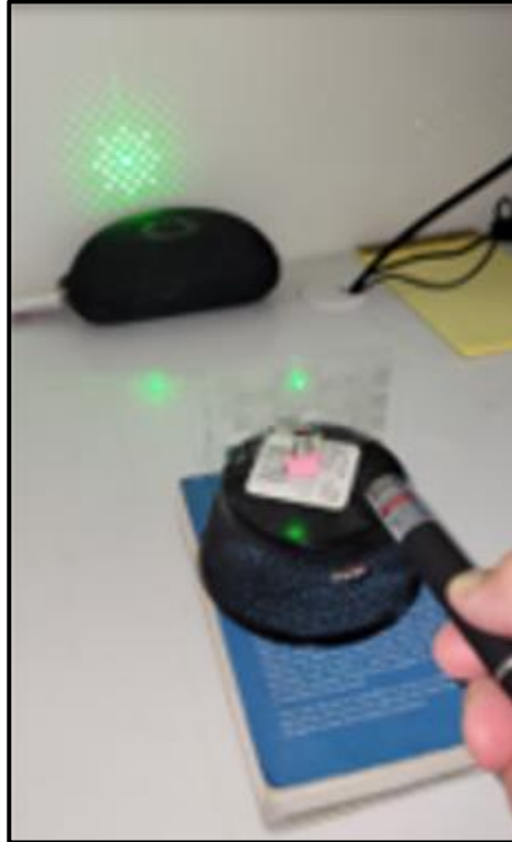
Figure 14. Photo from video that shows diffracted light patterns and images through the 24 custom diffractive optical elements.
