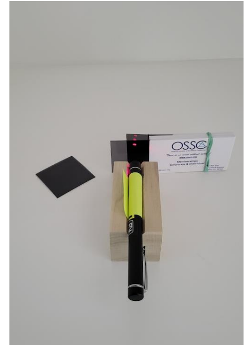
Laser with P(h+v) filters
