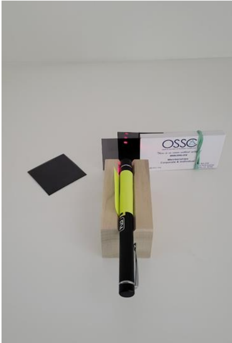
Laser with P(h+v) filters
