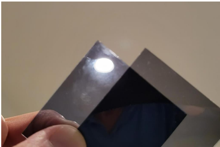
Ceiling light – one P(v) filter
