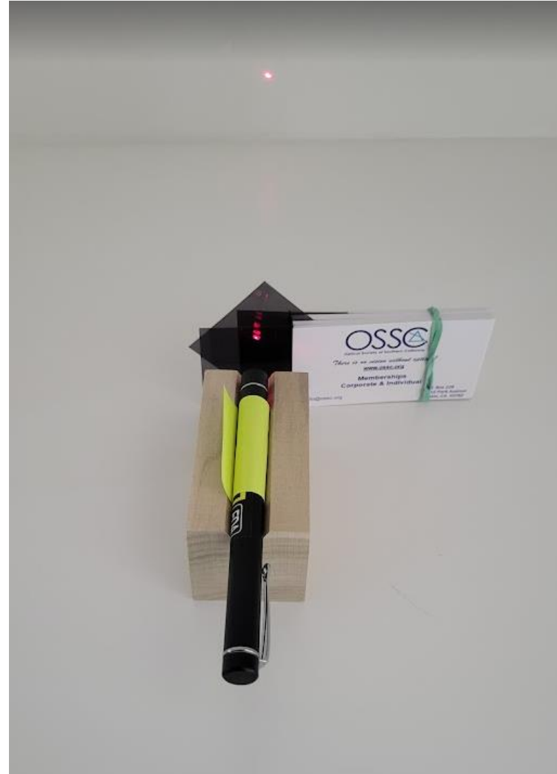
Laser with P(h+ v + 45) filters
