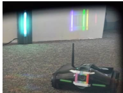
Figure 4. A high school student presents his work using a commercially available Rover 2.0 with a diffraction grating to demonstrate his knowledge of spectroscopy.
