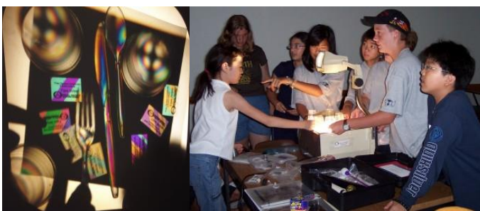
Figure 19. Young students use an overhead projector, two linear polarizers and plastic utensils to experience polarization.
