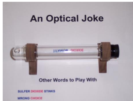
Figure 32. An ‘Alpha-Numeric Optical Inverter’ inverts the blue letters and numbers but not the red.
