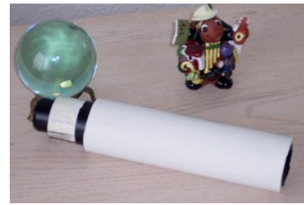
Figure 6. Fully assembled refracting telescope using glass lenses and PVC tubes.
