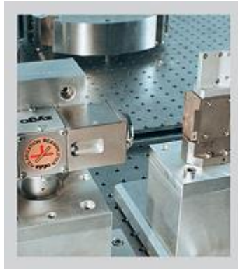
Figure 17. Typical distance measuring interferometer (DMI) used to measure closed loop position of a PZT system.
