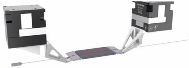
Figure 34. A model of special fixturing that is required to precisely align input and output optical fiber arrays to a waveguide.
