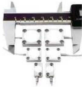
Figure 13. Example of capacitive sensors for position feedback; used in PZT stages and scanners.
