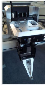
Figure 35. A photograph of special fixturing that is required to precisely align input and output optical fiber arrays to a waveguide.
